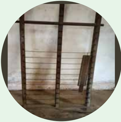
Creels: it is used to place the bobbins for the warping purpose
