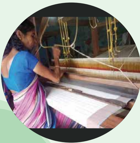
Smt. Bharathi Shettigar pulling the peg to control the shuttle movement using right hand. Simultaneously she pulls beater towards the fell of the cloth using left hand
