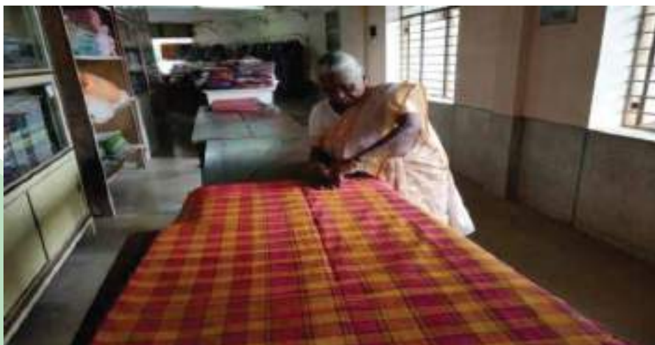
Smt. Mohini Shettigar at Kinnigoli checking the saree for broken yarns
