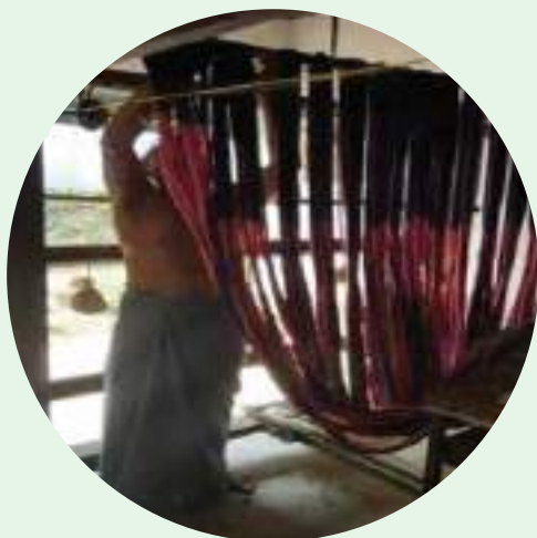
Arranging warp yarns over the loom
