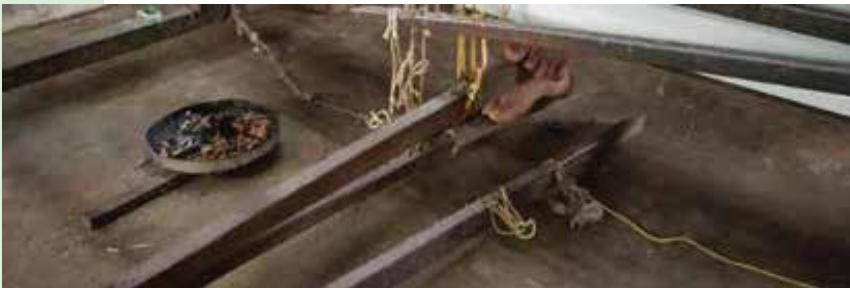
Treadles: controls Heald shaft
