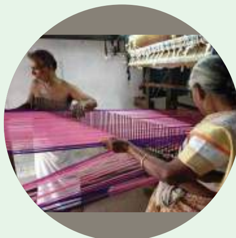
Passing yarns through raddle to avoid tangling
