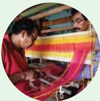
Shree Ananda Shettigar and Shree Venkatesh passing yarn ends through heald - drafting
