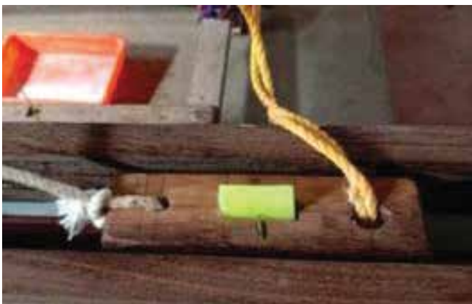
Picker: to push the shuttle
