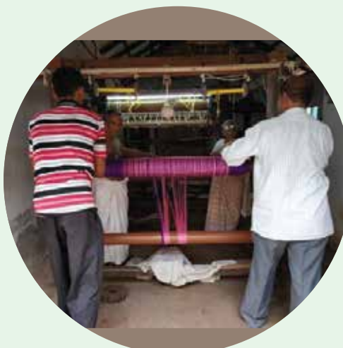
Winding yarns to warp beam – 5 persons required for this
