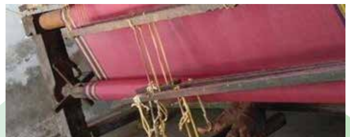
Cloth Beam: to wind woven fabric
