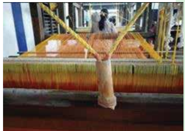
Peg to control the movement of shuttle
