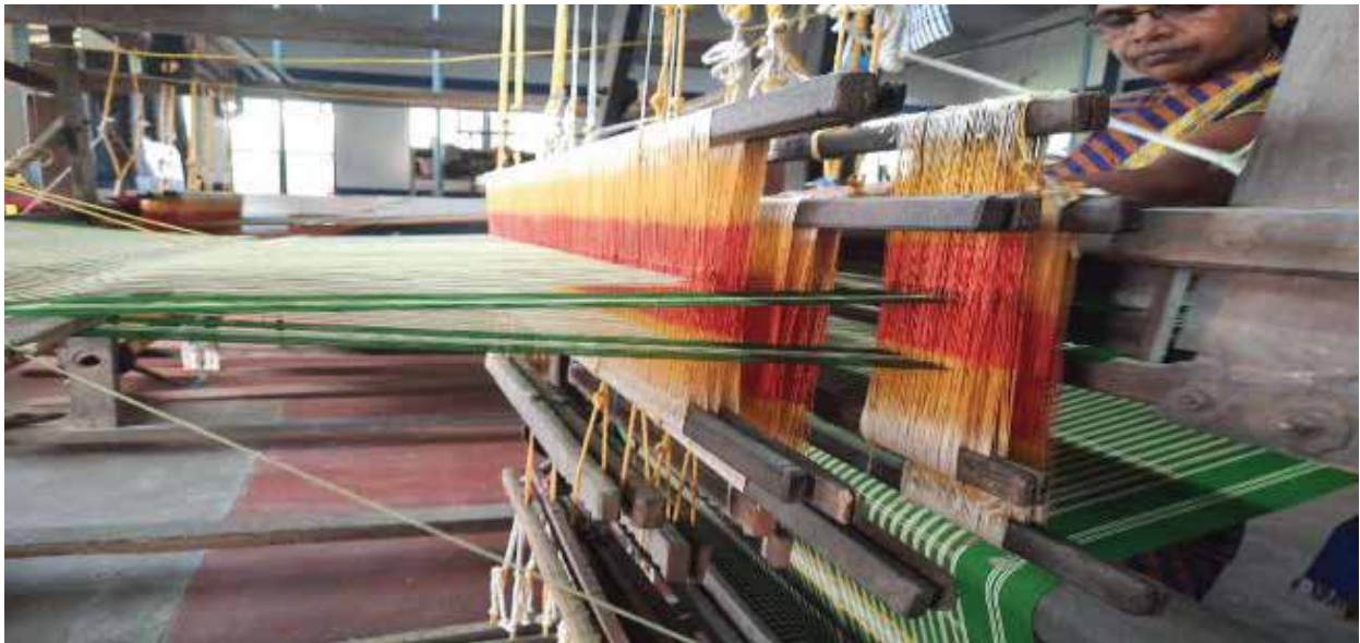
Smt. Vedavathi Shettigar weaving saree using cut border technique
