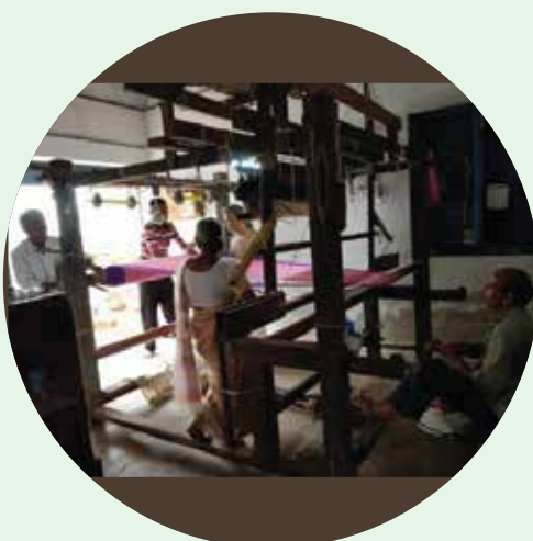
Winding yarns to warp beam – 5 persons required for this
