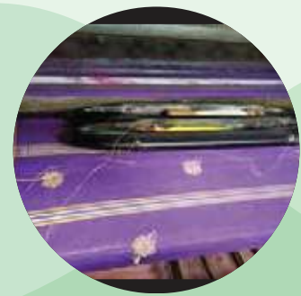
Extra weft yarns are inserted by hand using shuttle
