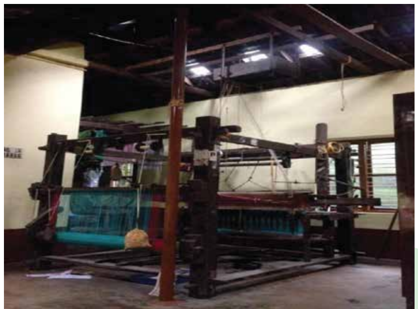
Malabar Frame Loom with sky light at Shree Harischandra Shettigar, Shirva
