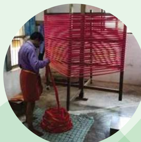
Unwinding yarns from the warping frame
